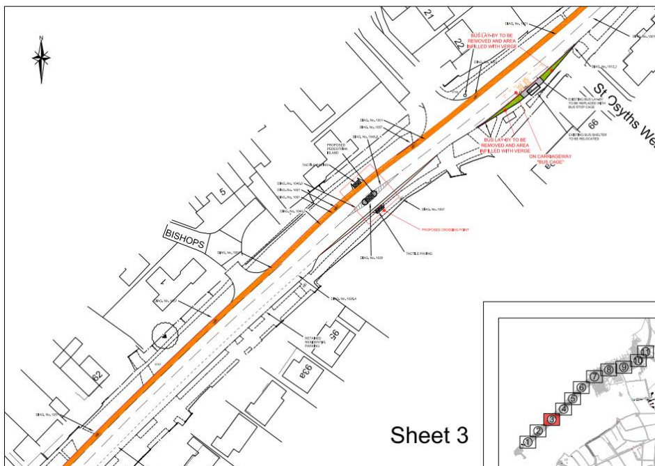
Figure 6: Off line to become on line bus stop and informal crossing point
